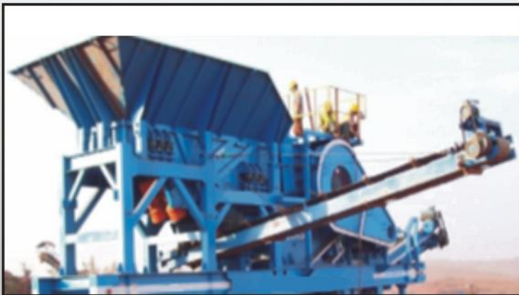
Second deck of Grizzly Feeder remove muck
